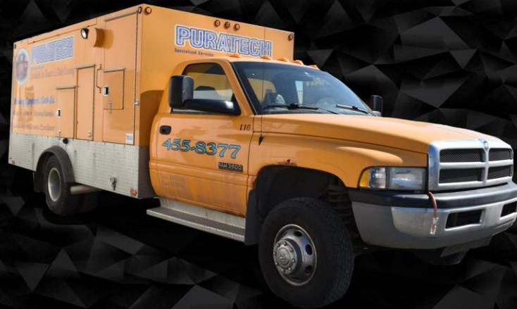
Lot 274 2001 Dodge Ram 3500, with 24 valve Cummins diesel engine, manual transmission, VIN 3B6MF36601M539895, 176,000km (2420 hours) with PTO drive to costume vacuum unit. Purpose built truck box has multiple locking storage areas to house required hoses and accessories. This estate unit was in operation up until this winter.
